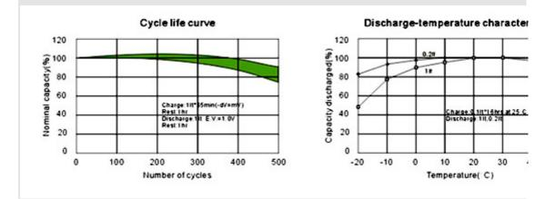
Cycle life Under normal conditions, 500-1000 charge/ discharge cycles can be expected.
